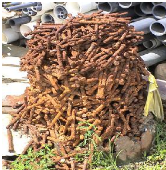
Steel bolts destroyed by rust
